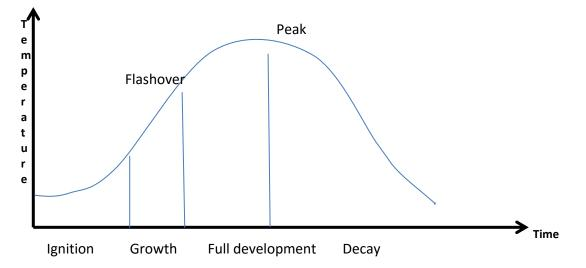
The flame retardant additives are active only in the first two stages of fire development.
